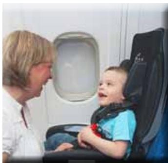
The TravelChair fits into a standard airline seat giving postural support for children. It is suitable for ages three to eleven, depending on size and weight. It has an adjustable headrest, footrest and body harness. The chair weighs 6kg and can fold to fit into an overhead compartment.
